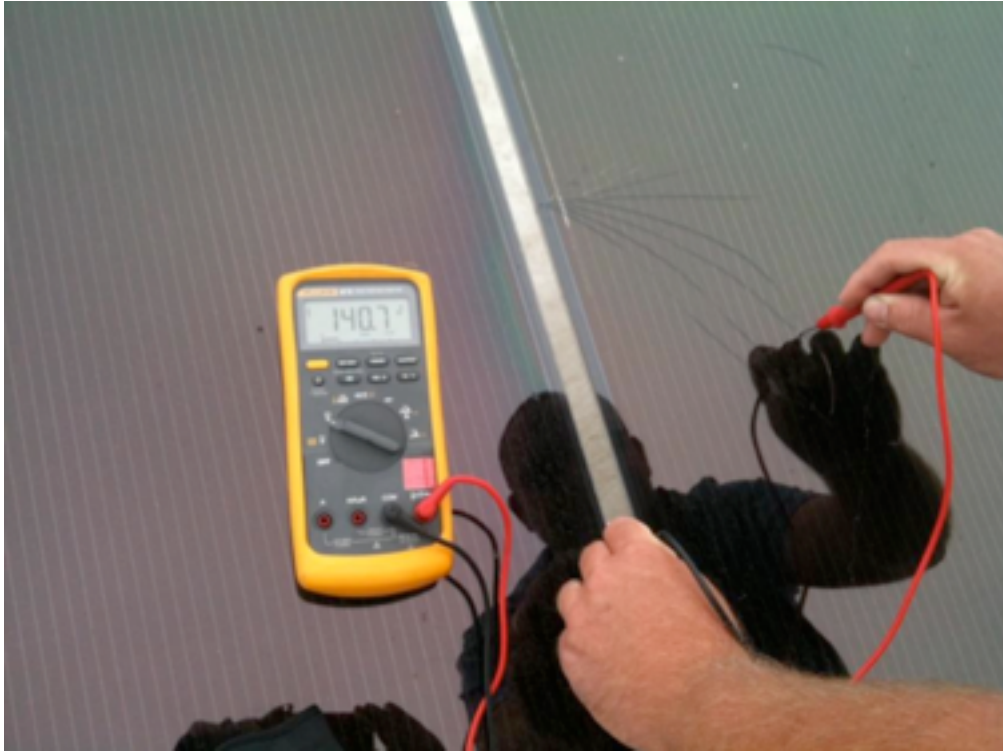
Fig.1: Example of measured potential between cracked front glass and rack.
